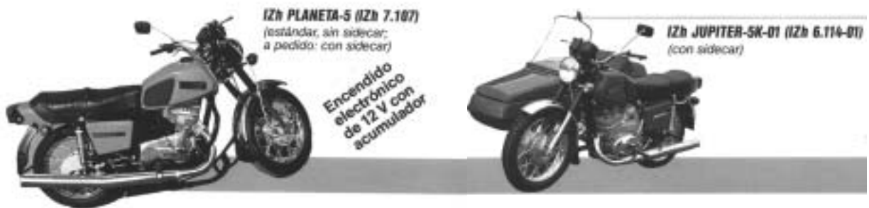
Planeta 5 and Jupiter 5 featured in Italian language brochure 1988 Planeta 5 – 346cc single two stroke 22 bhp 158kg 75mph
