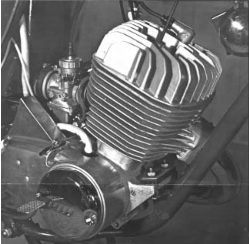
Left – the engine from the 1<sup>st</sup> version. Note the high quality finish to the die cast castings, the standard Mikuni carb and the rubber mounts at the front of the engine.
