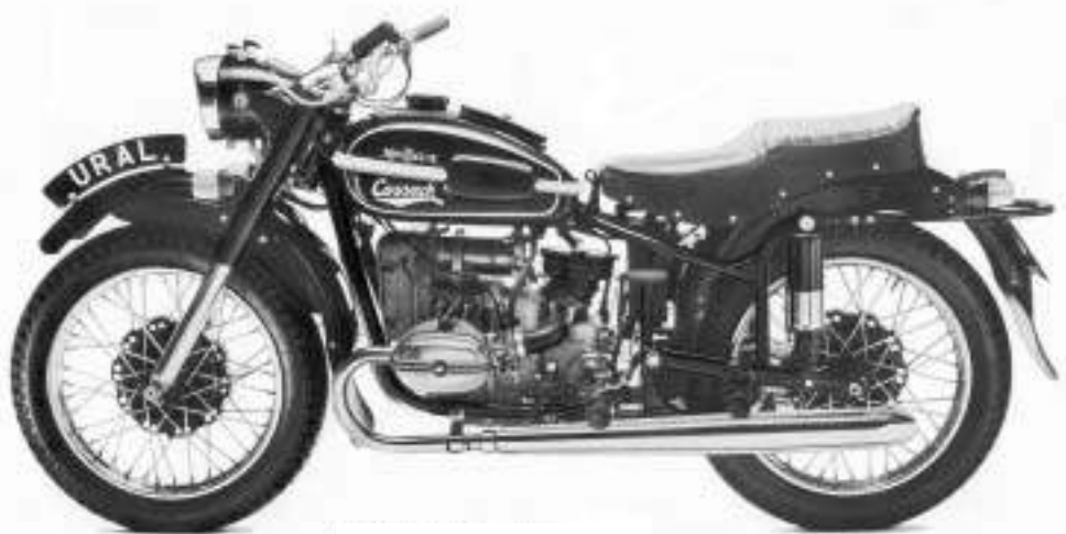
Ural M63, the first Ural to be imported commercially into England. Also note front mudguard as per M62 and introduction of the rear swinging arm.
