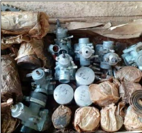
There's a lot more than pictured here, including cranks, gearboxes and most engine components. Yes those are cylinder liners on the left of the above picture, all wrapped up in Russian lanolin and brown paper. The porting would suggest a Champ is a
