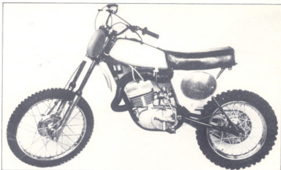
One of the special Soviet machines, only seen in the USSR. The 1978 Voskhod 250 motocrosser, with 36bhp, electronic ignition and monoshock rear suspension
