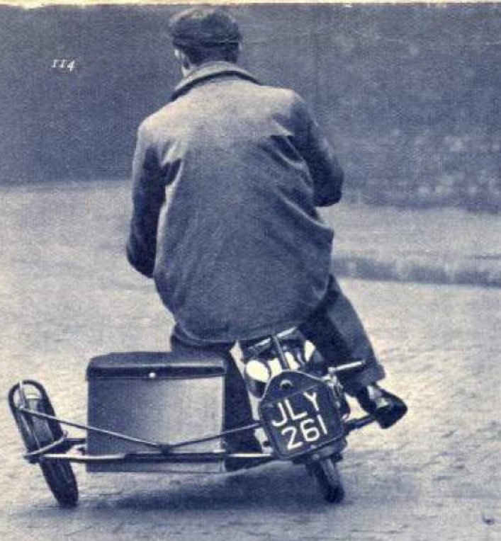
Cornering with the Corgi banking sidecar is as easy as with a solo. Note the tie-rod and slider mechanism, which controls the banking, at the rear of the sidecar
