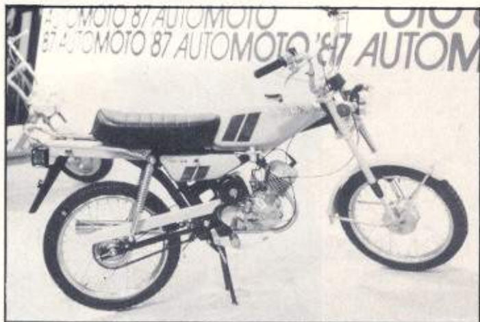
A 1987 Riga-24, an all-alloy two-stroke lightweight of modest performance.
