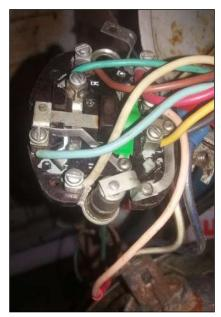
dark night. I have prepared my spare switch with soldered in tags which I will swap one day. Contact on main switch makes uncertain contact. Make sure it is clean and not touching
