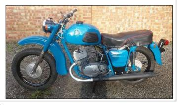
coarse but serviceable base. Fitting the Vostok replacement seat cover, (no holes for the pillion grip) was tricky, using some nice vintage style bifurcated rivets, especially as I had to allow for the extra thickness of the reinforced pan, but I think you will not notice too many creases in my picture on the previous page.
