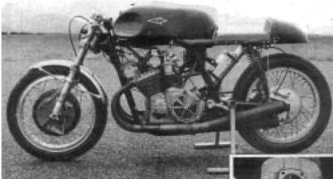
The Vostok 5-555 looked like a classic 1960s four — with duplex cradle frame and box section swingarm. And with development it might have been a threat to Ago and the MV Augusta.
