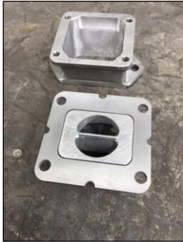
With a bit of welding and grinding the Yam reed fitted perfect and I used a reed stuffer to mate with the supplied inlet manifold. The carb from these bikes were copies of old looking Amal carbs, this engine will be running a more modern 60/70's Amal. As with tuning our Lambretta.
