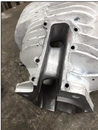
The 350 cylinder is certainly interesting as is the story of the manufacturer. The main strange thing was the sides of the transfer ports unscrew and come off, making transfer tuning a bit easier, but why I have no idea! Next was the twin exhaust ports! A simple way to widen the exhaust ports and gain some power. Our customer supplied a hand made reed manifold that he got from Ukraine, but that didn't fit the Yamaha YPVS 350 it was supposed to, so needed welding up, milling and grinding to suit.
