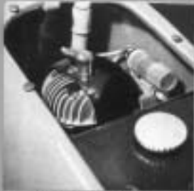
For filling or sparking plug checks, just swing away the saddle
