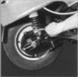
The rate of the scooter's rear suspension is easily adjusted for optimum running smoothness to load and road conditions
