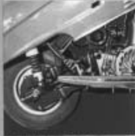
The final drive chain is made securely dust-proof with a housing and rubber casings
