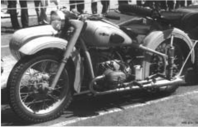
Ural M61, note plunger frame and front mudguard
